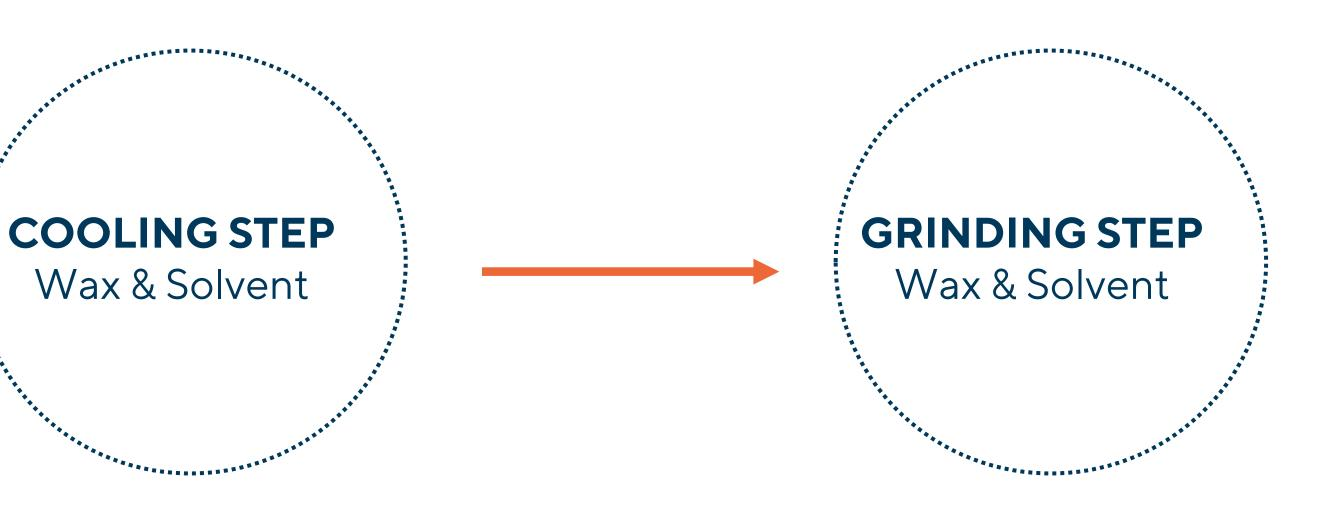
Once the system has cooled down and wax is well dispersed in solvent, there is the grinding step for achieving particle right distribution.
