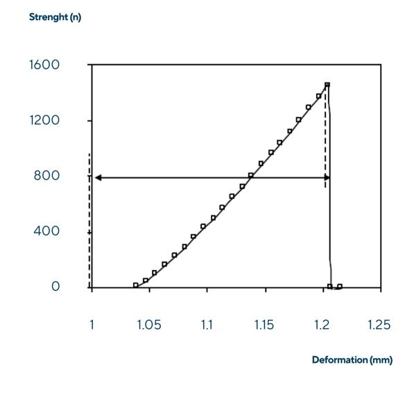
**Fig.3** Relationship between growing strength applied and the consequent deformation of the specimen.
