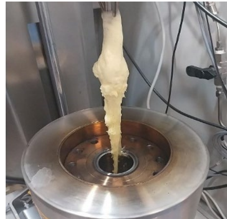
Figure 2: Polycarbonate obtained from mandarin oil and CO 2
