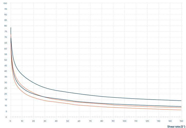
Standard engobe (density 1450 g/l, viscosity fc 4mm 12")
